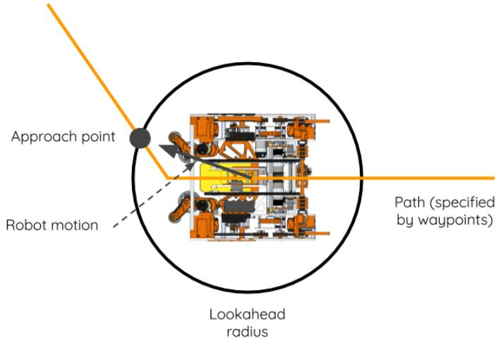
The general logic of pure pursuit is that we are dangling a carrot on a stick in front of the robot; the robot approaches not a set endpoint, but instead a “look-ahead” point that is a set distance further along the path than it. As the look-ahead point reaches and turns corners before the robot does, the robot begins turns early and thus rounds those corners.
